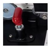
Cleat in locked position. beneath track flange and between track slots.
